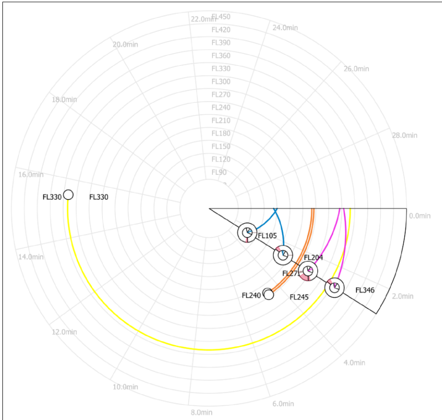
Figure 3.2: Improved visual encoding design of the TA display on the HTA-Viz interface. Based on the outcome of the qualitative study conducted with ATCOs both horizontal and vertical solutions to conflict were integrated into a composite glyph. To visualize the detailed information about solution spaces, ATCOs needed to manually zoom in on an aircraft glyph.
