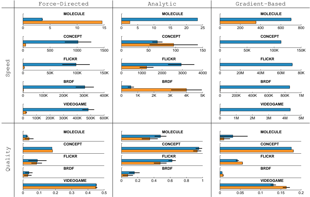
Figure 2: Comparison of speed (top) and quality (bottom). In each pair, the top blue bar is the original MDS algorithm, and the bottom orange bar is the Glint instantiations. The black lines indicate 95% standard error bars.
